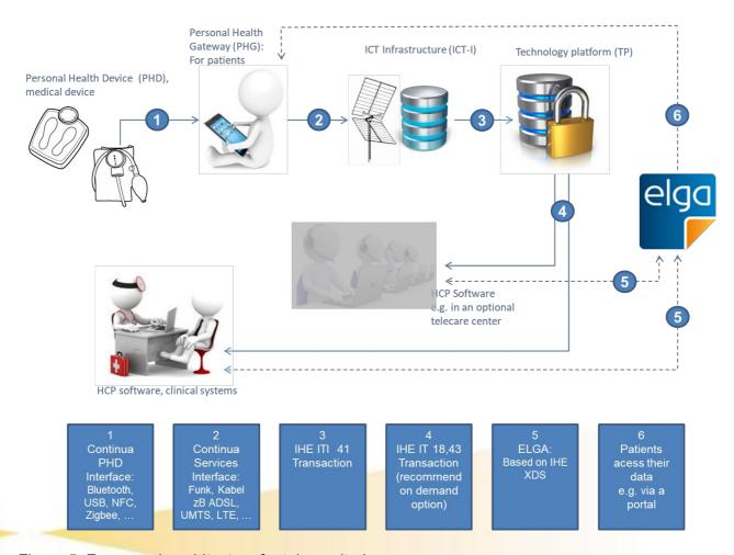
Figure 5: Framework architecture for telemonitoring.
