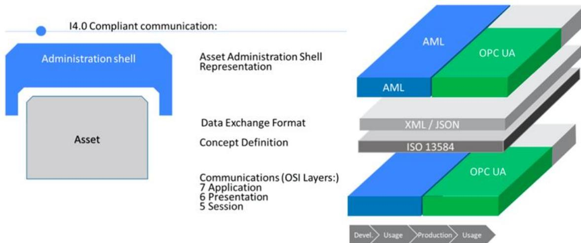
**Figure 19 – I4.0 Communication protocol stack**
