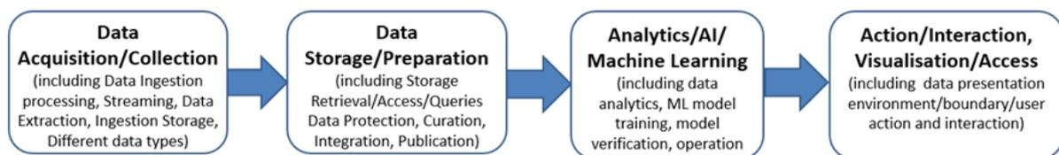
**Figure 24 – Top level Generic Big Data and AI Pipeline pattern**
