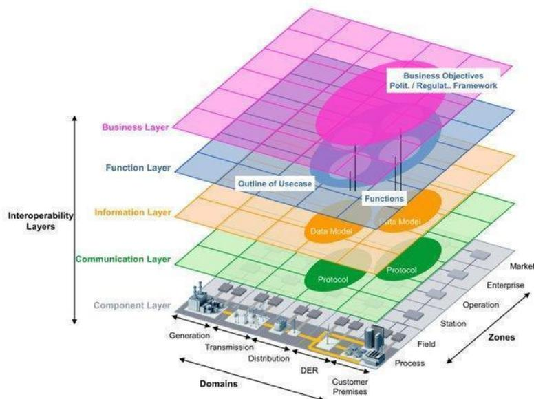
**Figure 33 – The Smart Grid Architecture Model (SGAM) Framework**
