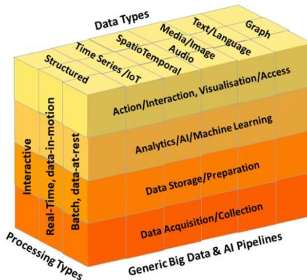
**Figure 25 – Top level Generic Big Data and AI Pipeline cube**
