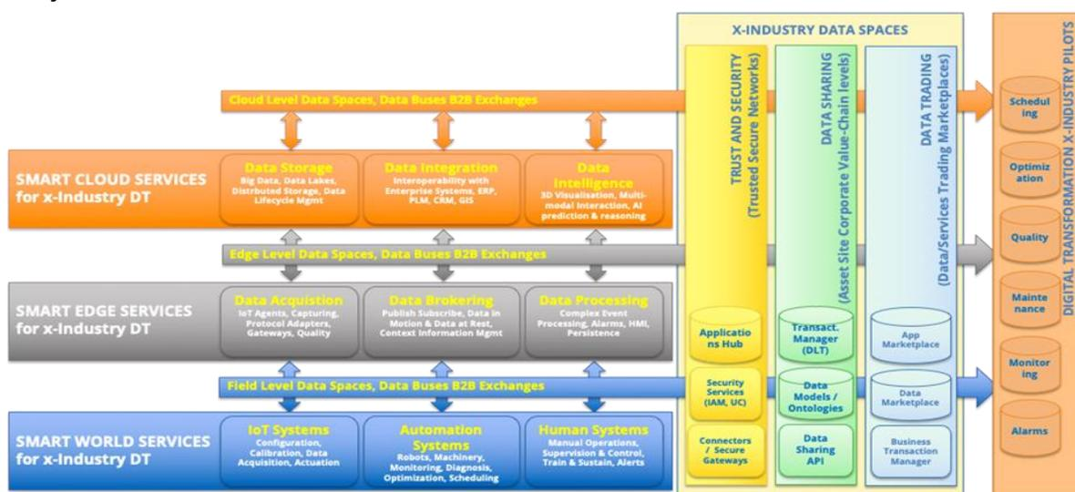
**Figure 1 – OPEN DEI reference architecture framework**
